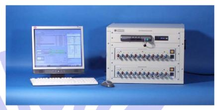
Three sections are easily connected together to maximize the throughput. The sections are networked together using a high speed multi-port Ethernet switch so that all sections may share a common control window. Once a duplication job is launched in the user friendly GUI window, each section is individually started using the sections' START Key.
